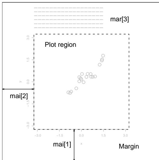
**mar** A numerical vector of the form `c(bottom, left, top, right)` which gives the number of lines of margin to be specified on the four sides of the plot. The default is `c(5, 4, 4, 2) + 0.1`.
